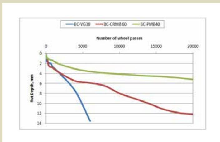
Figure 3 Hamburg Wheel Tracking Test @50C
