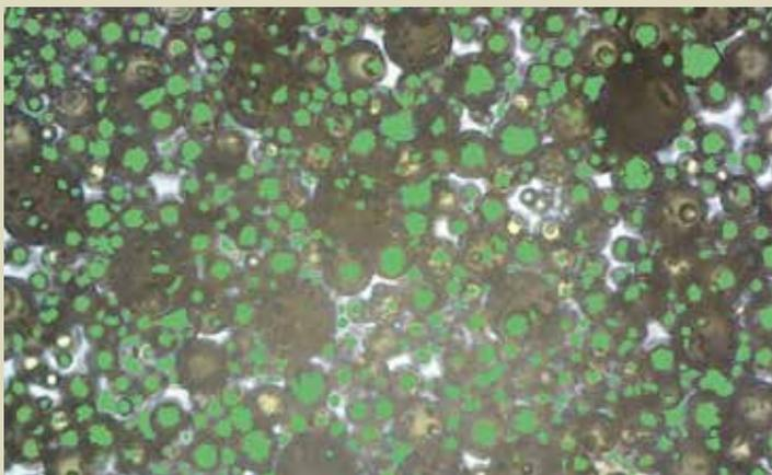
Figure 1 Microscopic View of Bitumen Emulsion
