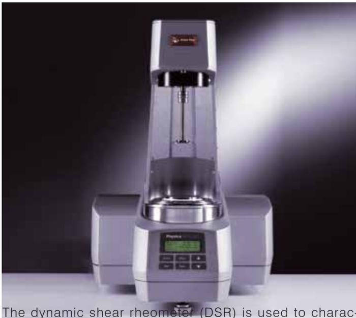
The dynamic shear rheometer (DSR) is used to characterize the viscous and elastic behavior of bitumen binders at medium to high temperatures. This characterization is used in the Superpave PG bitumen binder specification. As with other Superpave binder tests, the actual temperatures anticipated in the area where the bitumen binder will be placed determine the test temperatures used.
